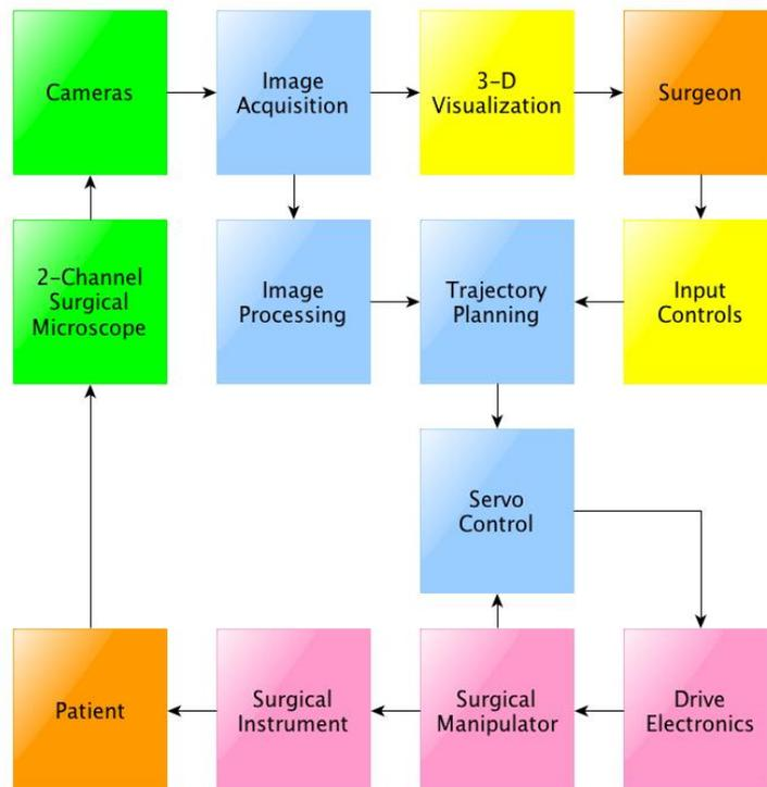
With the aid of an optical tracker that provides positional feedback, it is possible to improve the surgeon's decision-making and interpretation of data. One suggestion for an optical tracking system is to attach a camera to the surgeon's microscope. This approach
