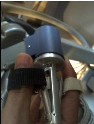
Figure 2: da Vinci right-hand side tool manipulator at the master's console. Tool manipulators allow the surgeon to control the tools held by the da Vinci's arms at the slave side.
