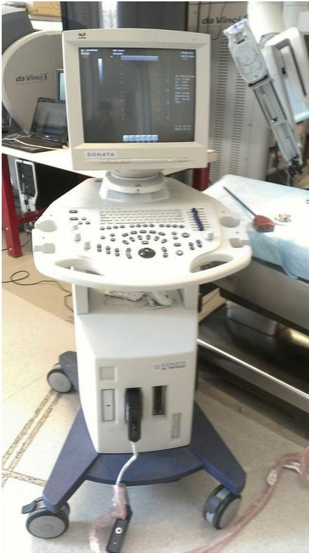
Figure 3: Mock OR testing setup. In the forefront is the ultrasound machine used to grab live ultrasound feed from the probe and transmit it to the laptop and the TilePro interface. Left and in back is the master's console, and to the right is the slave side complete with the operating table and equipped da Vinci robot arms.
