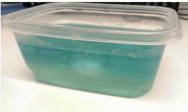
Figure 5: Gelatin phantom. An white agarose/glycerol pseudolesion is visible at the center of the phantom.
