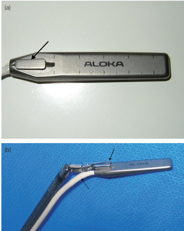
**Fig. 1** (a) Robotic ultrasound probe used for tumor identification during RPN. The robotic ultrasound probe has a grooved ridge on its ventral aspect (solid black arrow) that fits the robotic grasping instrument. (b) Robotic ultrasound probe with notch attached to robotic instrument (solid black arrow). The probe has a flexible cable (dashed black arrow) that allows passage through the assistant port and allows for full articulation of the robotic instrument.
