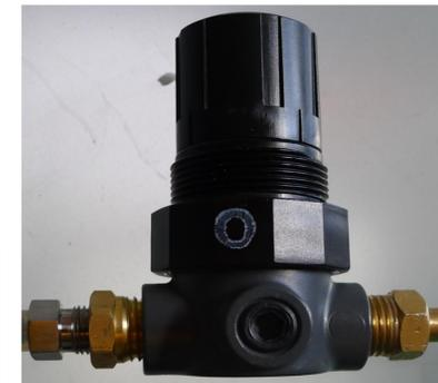
Fig. 2 Pressure regulator valve
