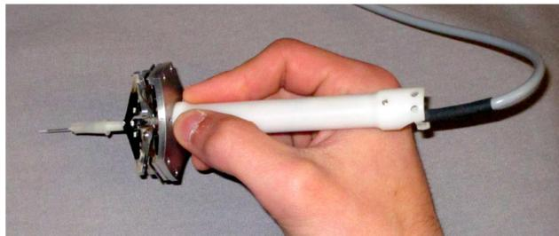
Fig. 1. Micron micromanipulator without casing to illustrate the piezoelectric motors between the handle and tip of the instrument, which enable the tip to actuate independently of the handle (or hand) motion.
