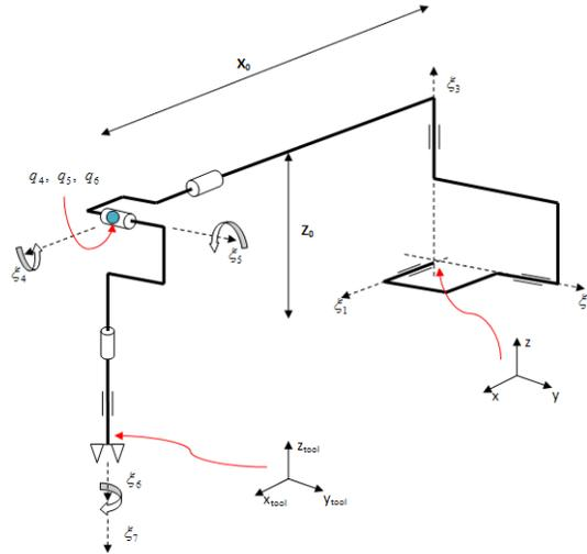
Fig 5. Twists assigned to the robot joints.[3]
