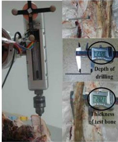
Depth measurement before and after drilling through the bone
