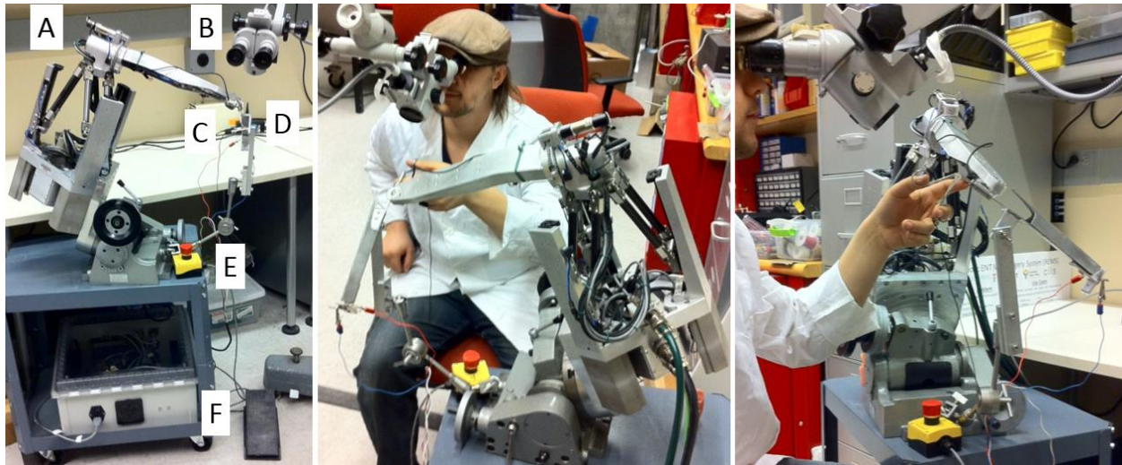
Fig. 1. Left: REMS Overview: A) Robot B) Microscope C) Laryngeal instrument D) Phantom mounted to training laryngoscope E) Emergency stop button F) Robot control pedal. Middle/Right: Example setup of REMS in use
