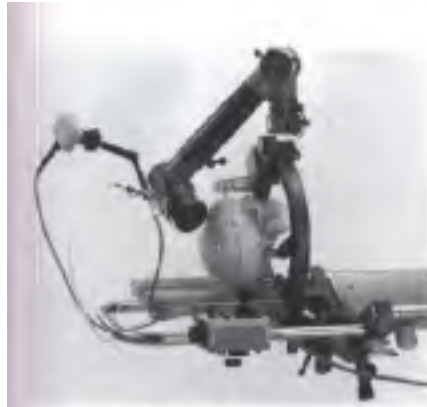
Figure 23.6: Digitizer of the second generation with video microscope and docked video camera. (Center bottom) Control console.
