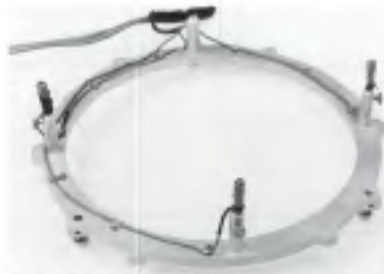
Figure 5. Sonic emitter ring, which attaches to the DMT head ring by the standard DMT head/scan disk system; connectors can be placed on four points around the ring, allowing its use for posterior-based craniotomies.
