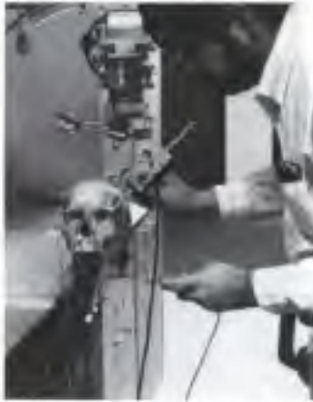
FIGURE 10.11 Tracking headsets on the skull. The position of the tip of the distal end of the handpiece on the skull has previously been calibrated. The positions of the beacons mounted in the skull are rigorously maintained to provide a base coordinate system for the handpiece location. Once the skull has been located, the position of the beacons relative to the preoperative skull coordinate system may be compared.
