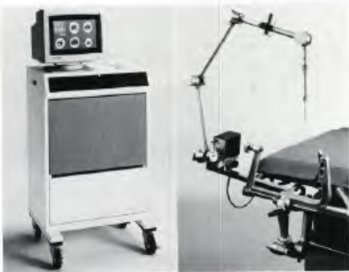
Figure 2. Photograph of the neuronavigator. The computer station is located in the console area on the left. The viewing arm is secured to the Mayfield skull clamp. Six CT slices are displayed on the computer screen. The cross markers display the location of the navigators tip.
