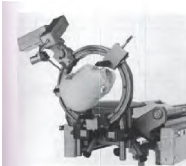
FIGURE 23.4 The ET-01 measuring arm with 4.5 degrees of freedom.
