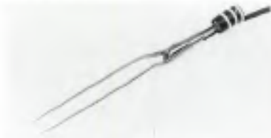
Figure 4. Sonic forceps, with wires directly attached to the handles since the designs involved precluded the use of a conventional connector.
