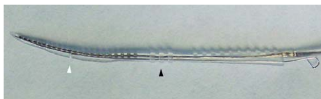
Fig. 1 Contour Advance electrode (Cochlear Ltd.) with soft tip is a preformed electrode carrier pre-operatively straightened by a platinum wire (stylet). A white marker ( white arrow ) and ribs at the end of the electrode carrier ( black arrow ) give orientation for the surgeon during insertion. A loop at the end of stylet allows coupling to the insertion tool
