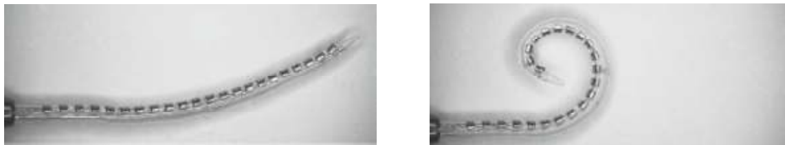
Figure 3 - Cochlear Nucleus 24 Contour Advance Practice Electrode. After stylet retraction, the array turns to its preformed state [11].
