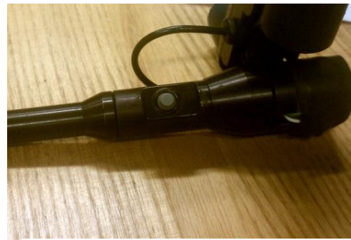
Figure 5: The PHANTOM Premium stylus, complete with button
