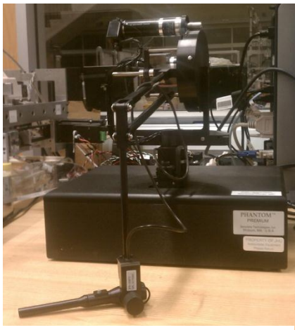
Figure 4: The PHANTOM Premium haptic controller
