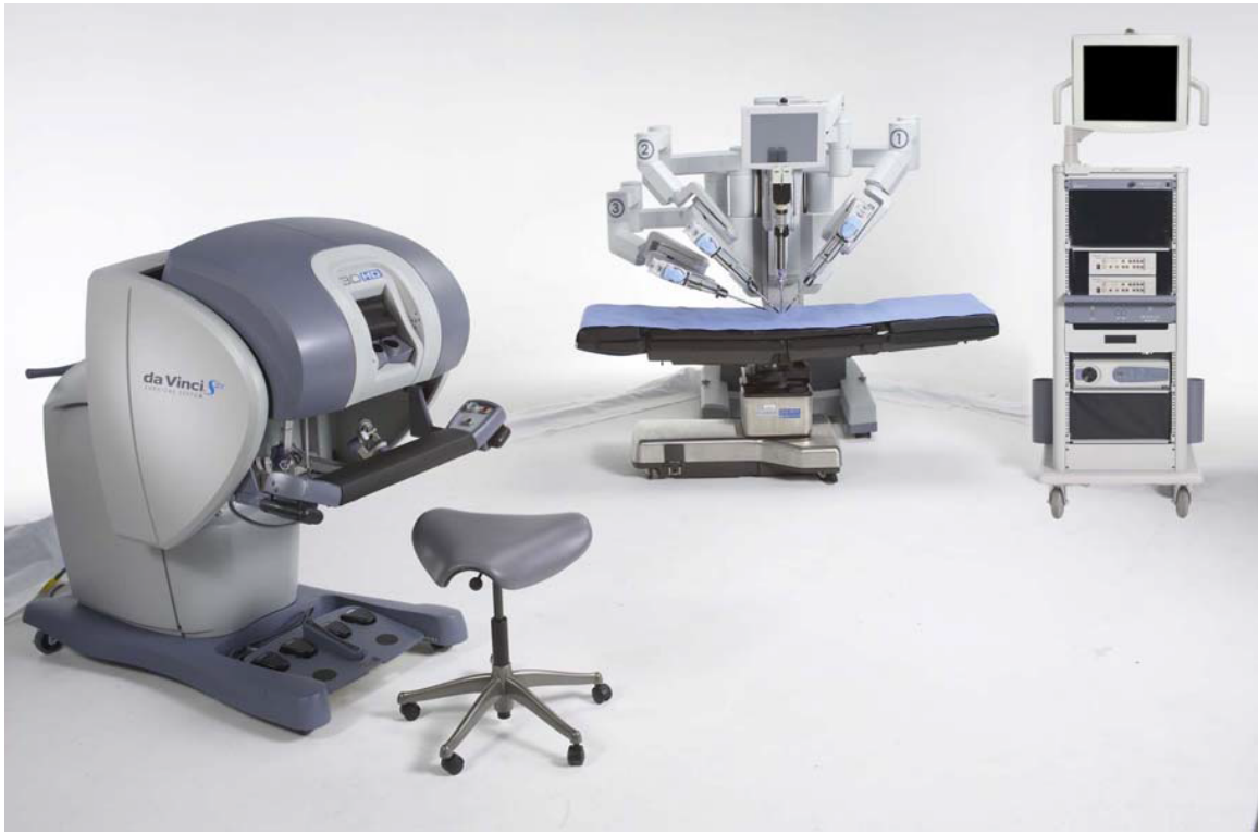
Figure 1: daVinci S System setup - (from left to right) Surgeon Console (Masters), Patient Cart (Slaves), Vision Cart.
