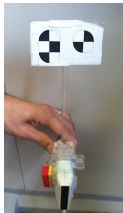
Figure 4. Freehand ultrasound probe holder and ring
