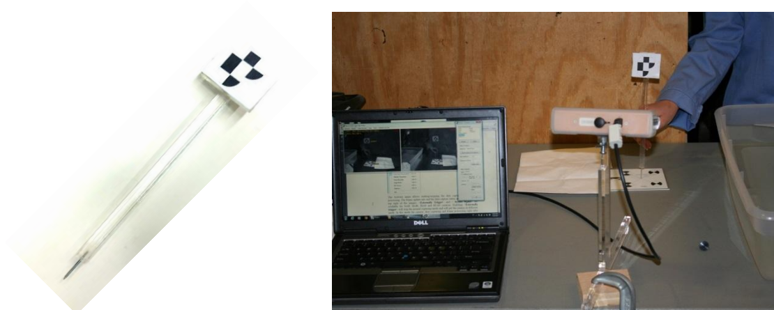
Figure 7. Pointer and its calibration procedure using MicronTracker
