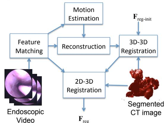
**Figure 4:** Motion estimation and registration chain implemented during prior R21 grant.
