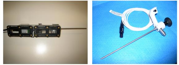
**Figure 9:** Left, a high-precision optically tracked endoscope developed for cadaver data collection and algorithm validation. Right, a more recent EM tracked scope for use in airway data collection.
