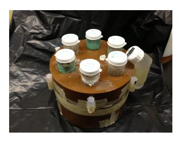
Cylinder phantom that contains varying iodine concentrations.
