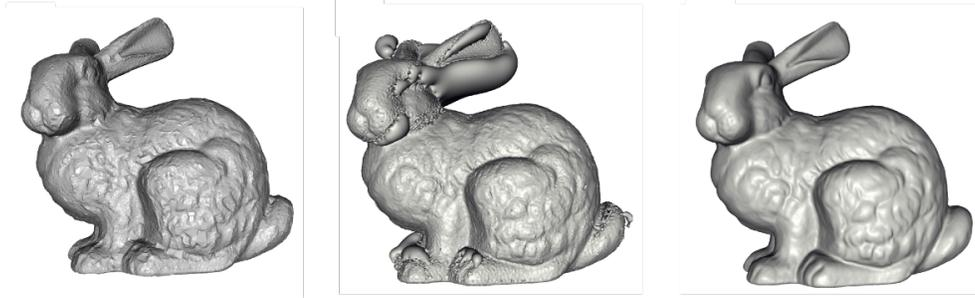
Figure 5: Results of surface reconstruction for the “Stanford Bunny” dataset. The left shows reconstruction using Robust Cocone method, the center shows reconstruction from the Fast RBF method, and the right shows reconstruction using the Poisson method. (Graphics are from [9])
