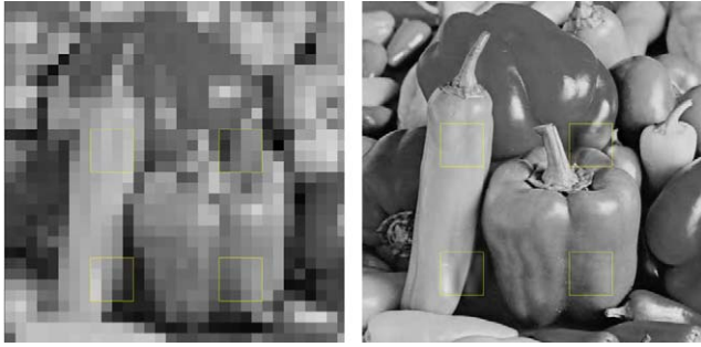
Fig. 7. Concealment of four packet losses in the lowpass band. Left: Lowpass with errors concealed. Right: Reconstructed image with errors concealed.
