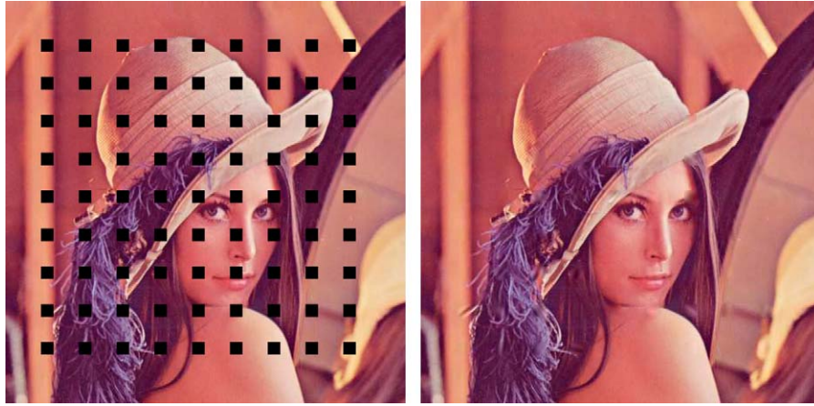
Fig. 5. Concealment of block losses using the frequency selective extrapolation technique. Left: Isolated 16 \times 16 block losses. Right: Concealed image.
