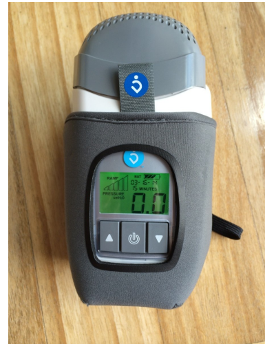
Figure 5: Z1 portable CPAP device (Mistatic.com)
