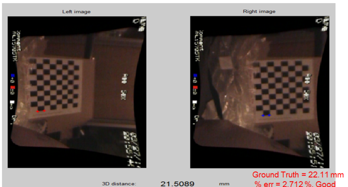
Figure 4. Measurement of the 3D distance of an artificial scene.
