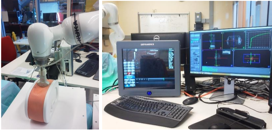
Figure 5: KUKA Robot with ultrasound phantom and workstation running ImFusion during the visual servoing experiment
