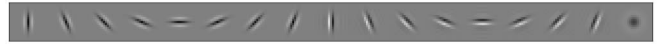
Fig. 5. Filters for creating textons. We use eight oriented even and odd symmetric Gaussian derivative filters and a center surround (difference of Gaussians) filter.
