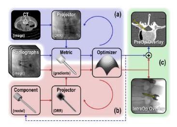
Uneri et al. employs a similarity metric based on pixel-wise correspondence of gradient intensity. Shown below are the equations that define said metric. Given that f is the fixed radiograph, m is the moving DRR, and (i, j) denote 2D image pixel coordinates, the method seeks to maximize the gradient correlation between a fixed radiograph and some DRR.
