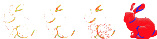
Figure 4: FPFH persistence of varying radii from r = 0.003-0.005 cm as well as overall points
