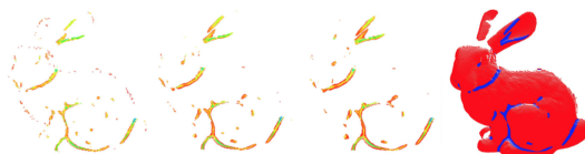
Figure 2: PFH persistence of varying radii from r = 0.003-0.005 cm as well as overall points
