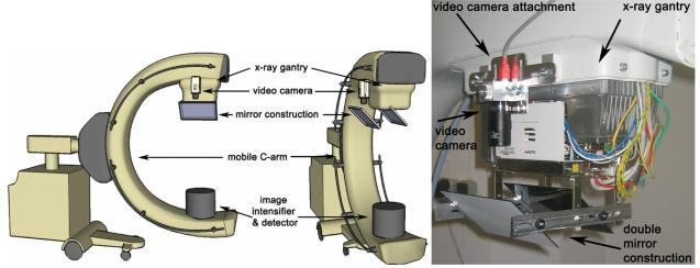
The C-arm used is a Siremobile Iso-C 3-D from Siemens Medical Solutions, and the video camera is the Flea from Point Grey Research, Inc. connected by a Firewire connection. The mount and mirrors construction was custom made.
