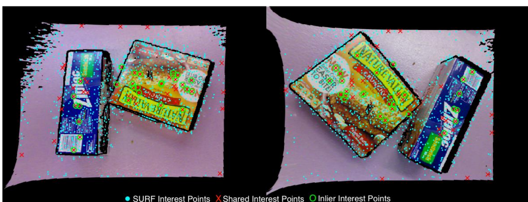
Fig 5: Two images of the same calibration scene taken by the two robots, with SURF features marked.
