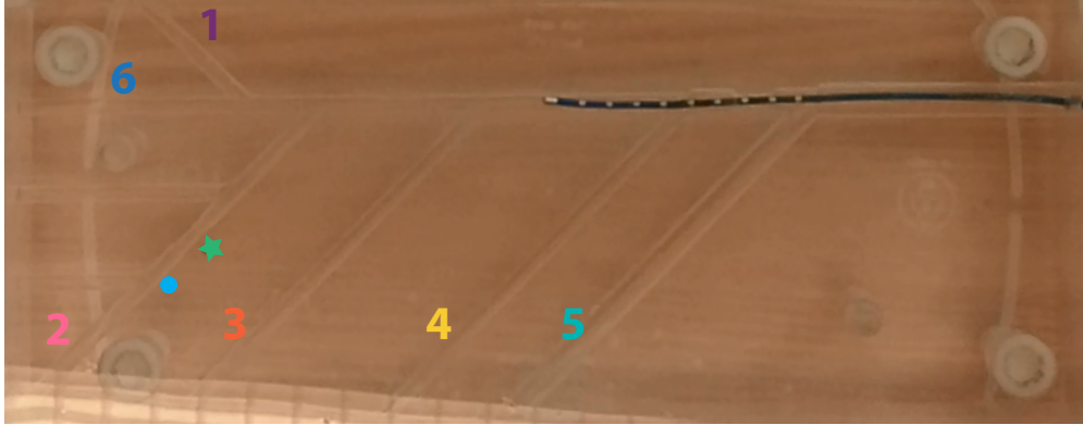
Figure 9: Synthetic phantom with labeled paths. The two halves of the phantom were machined from acrylic and sealed with a thin layer of transparent waterproof grease. When assembled, it measures 10\text{ cm} \times 25.4\text{ cm} \times 5\text{ cm} . The paths are 2.5-10 mm diameter.
