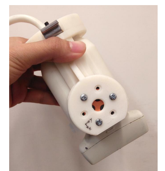
Figure 9. US attachment with 3-axis load cell
