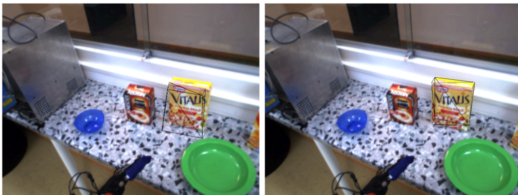
Figure 4 – Result of 6-DoF pose estimation. Left: monocular approach (when it is instable); Right: Stereo-based approach.
