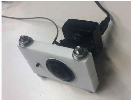
Figure 1. Mechanical setup of the camera and laser, using a 3D printed frame.
