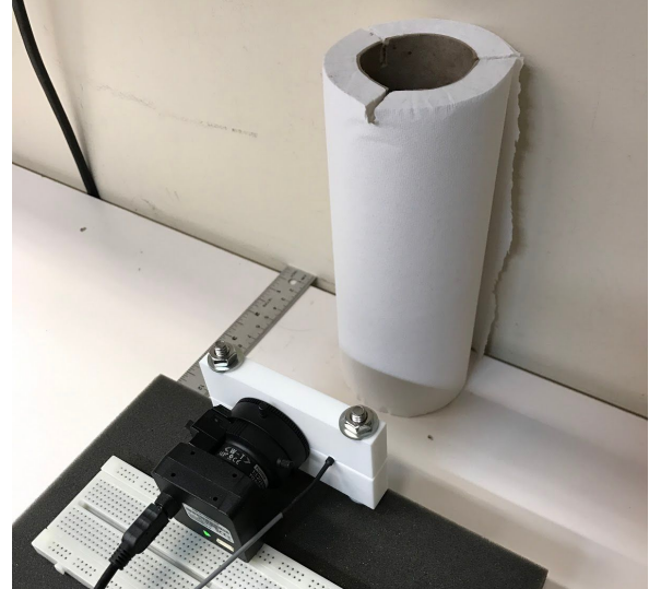
Figure 8. Real world x and y coordinates of cylinder at 80-160mm away and image of setup.
