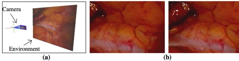
**Fig. 3.** An illustration of the simulation environment used to generate a stereo-laparoscopic video with known ground truth data for camera motion. A 3D rendition of the virtual world is shown in (a) and an example stereo pair taken from the virtual cameras is shown in (b).
