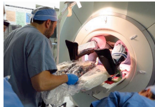
Slide in robot until hit Z-frame
