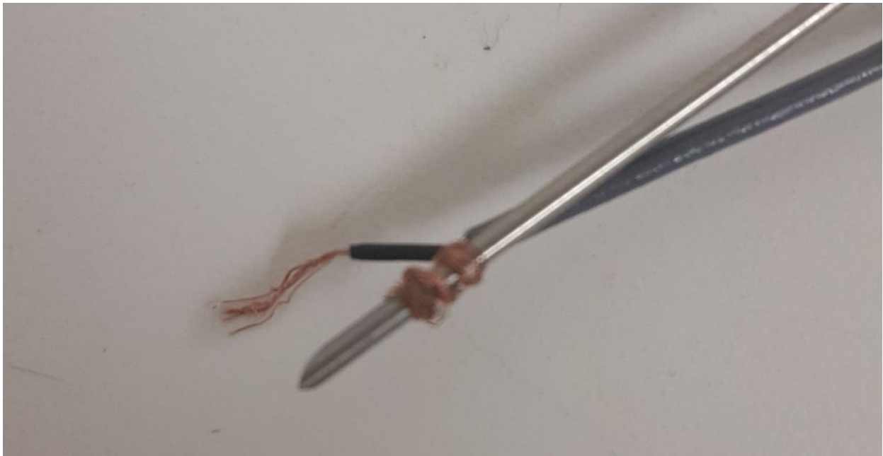
Wrapping the ground wire around the needle at the tip.
