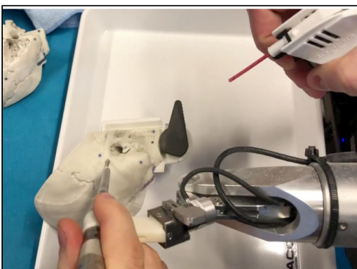
Figure 2: Galen and surgeon cooperating while drilling a mastoid bone[2]
