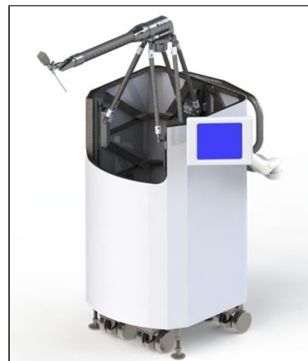
Figure 1: Full assembly of the Galen Mk. 2 platform [1]
