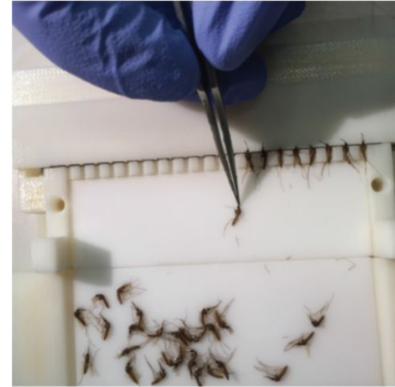
Figure 4. Semi-automatic Mosquito Micro-dissection System (saMMS) (Schrum)
