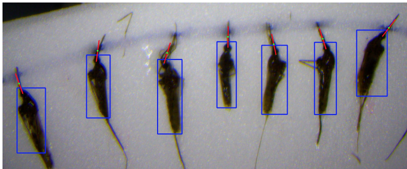
Sample results: mosquito & proboscis finder. Blue boxes indicate detected mosquitos, red lines indicate detected proboscises
