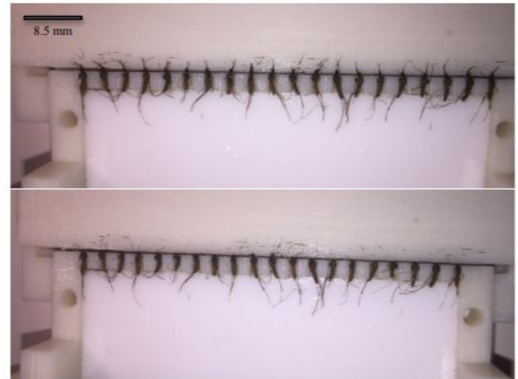
Fig. 4. Decapitation. (Top) Mosquitoes aligned in cartridge with heads between decapitation blades. (Bottom) Mosquitoes after decapitation.
