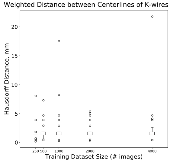
Figure 10: Hausdorff distance to centerline as a function of training dataset size. Differentiation between training set sizes is more limited indicating that for the portion of K-wire detected, the path of the K-wire is accurate.
