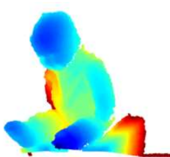
Figure 1: (Left) Depth map of a baby doll (Right) RGB image of a baby doll (Provided by Group 15)
