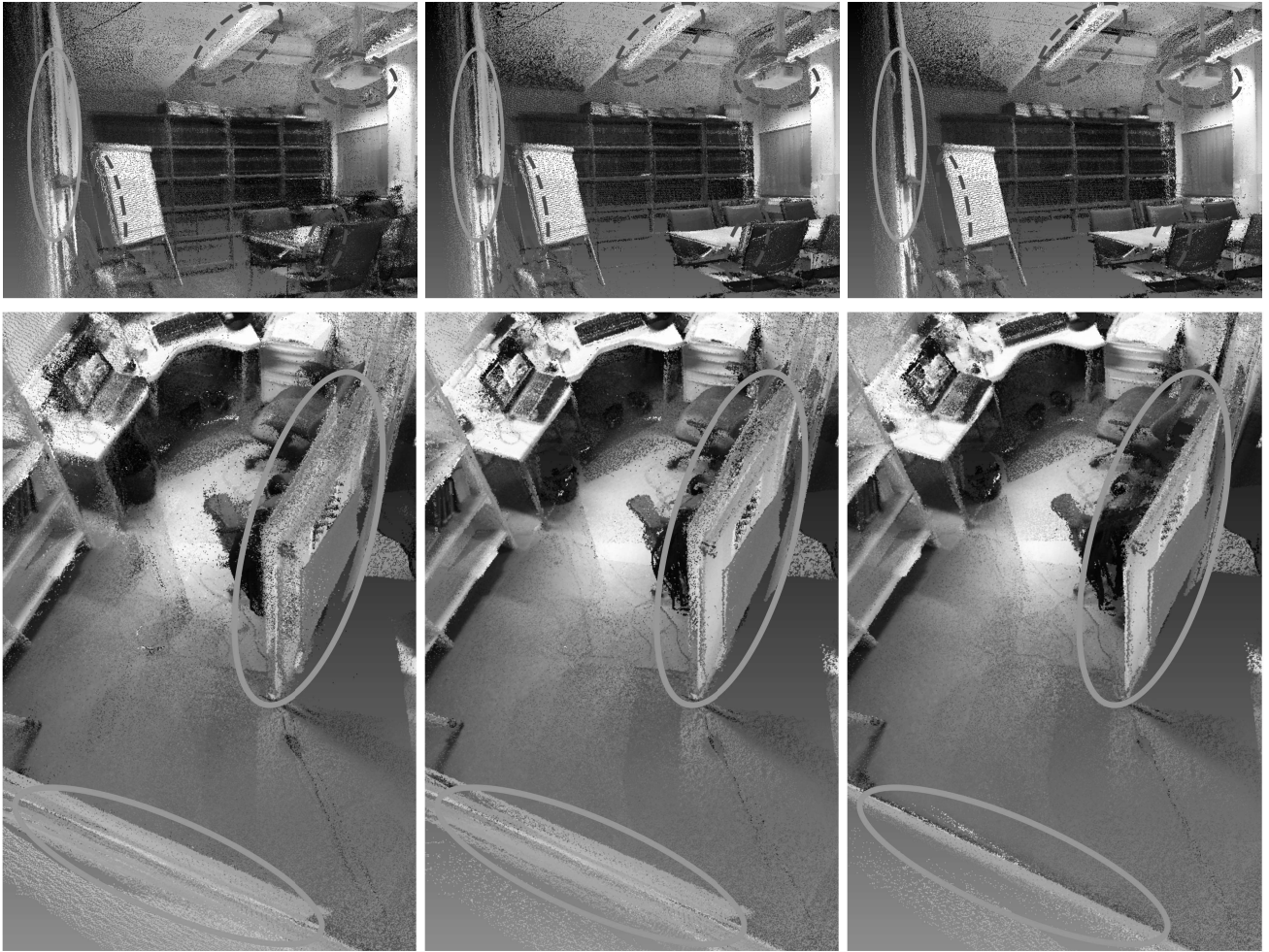
Fig. 5. Comparison between Office1 (top) and Office2 (bottom) results made with the methods in [11] (left) and [12] (middle) and with the method proposed in this paper (right). The proposed method significantly reduces the amount of registration errors which makes the surfaces less ambiguous (green ellipses) and the object boundaries more accurate (red dashed ellipses).
