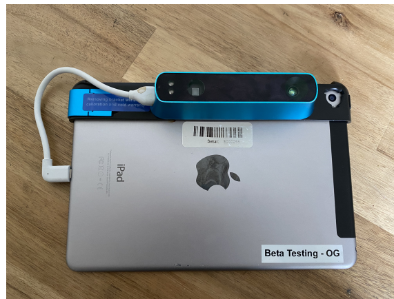
Figure 2: Structure Sensor attached to an iPad, provided by PediaMetrix.
