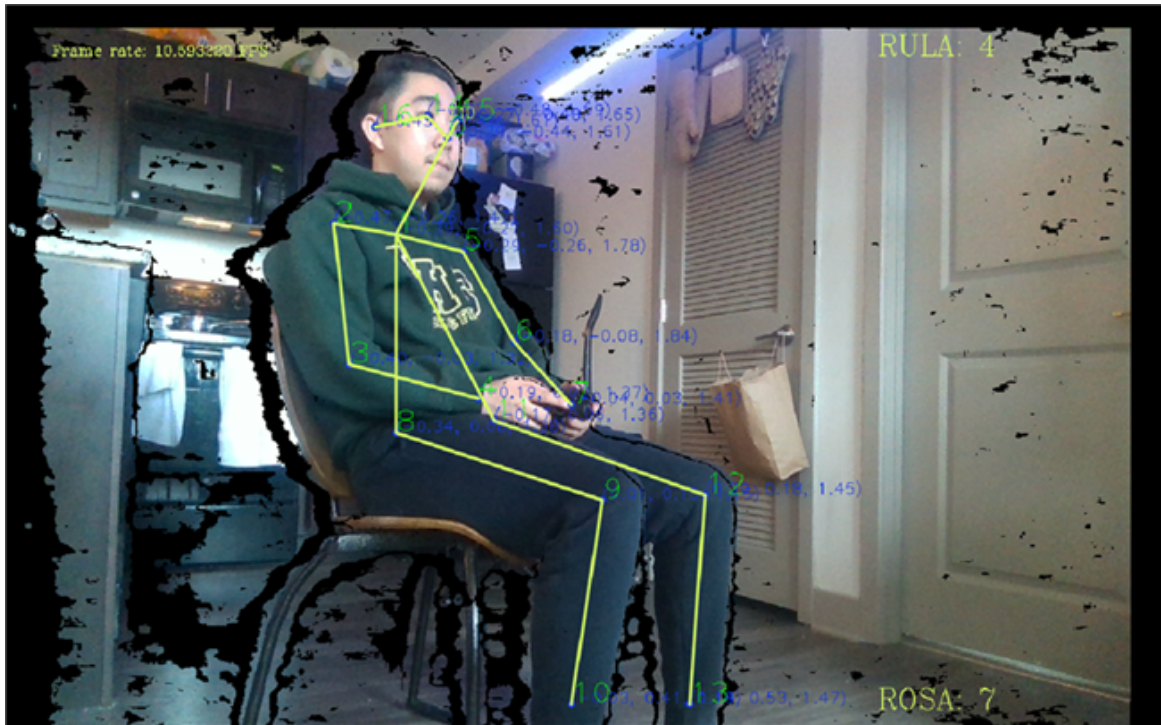
Figure 2: Screenshot displaying joint ID and position, real-time RULA (upper right) and ROSA scores (lower left)
