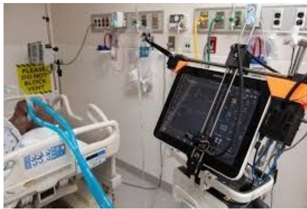
Figure 2. The 2D Cartesian robot designed for controlling touchscreen (JHTV)
