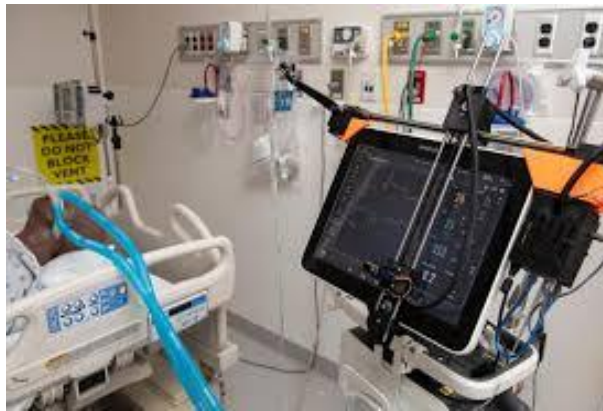
Figure 2. The 2D Cartesian robot designed for controlling touchscreen [1]
