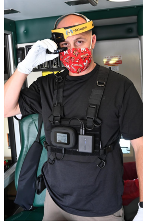
Dr. Nick Dalesio of JHU in an ambulance, wearing smart glasses on a medical head mount. On his chest are a MiFi unit for mobile broadband and an auxiliary battery.
