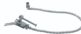
Figure 4: Flexible snake arm. The base of this structure is clamped onto a patient's hospital bed or retraction system mounted around the patient's head. A tool used in the brain is clamped to the opposite end of the arm. The arm is curved in the surgeon's preferred shape. The middle knob is tightened and the arm becomes rigid.
