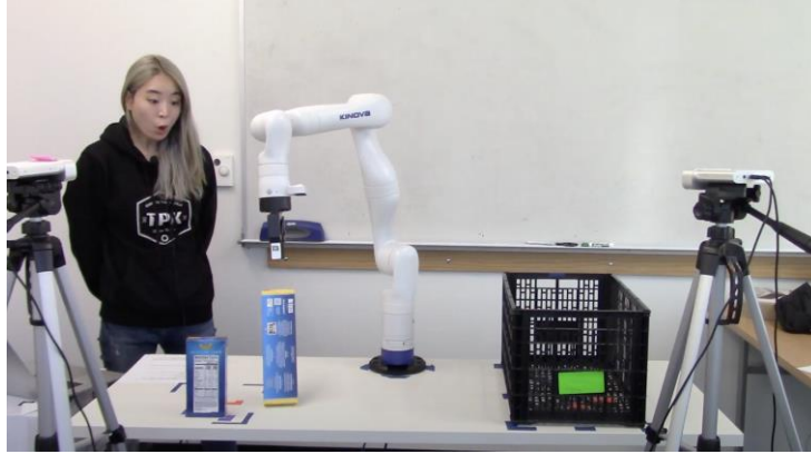
Figure 1: Sample reaction from Stiber pilot study. The image also shows the technical setup of the cameras used for AU detection.
