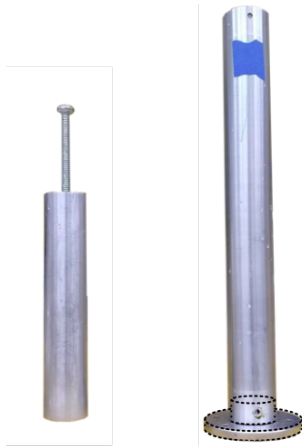
Figure 6: Plunger (left) and tube (right) used to create samples. The detachable bottom plate (black dotted) can be attached to either end of the tube. The taped end is slightly looser than the non-taped end. The tighter end is for forming the overall shape and a uniform bottom surface, while the looser end is used to remelt top portion of the sample in order to create a uniform top surface. The plunger is used to push the sample out of the tube, and to apply pressure during the remelting step.
