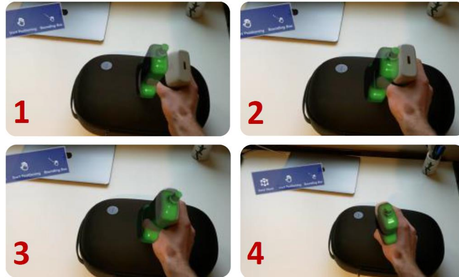
Fig. 3. Follower-Side Interface and Teleoperation: The follower sees the virtual transducer and a control menu. In frames 1-3 the follower starts in a random position and matches the virtual probe pose precisely within < 0.5 sec, before the probe pose changes and is immediately matched by the follower again in frame 4. The transducer is green to indicate the expert is happy with the applied force.
