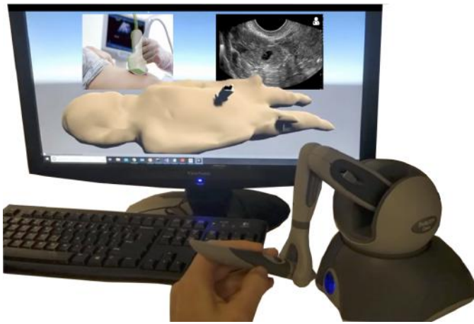
Fig. 4. Expert Workstation: the Phantom Omni haptic controller (front) is used to input pose and force and provide haptic feedback. The virtual probe relative to the patient mesh is visualized with the live ultrasound images and MR capture video call shown above it.
